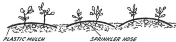
Fig. 8. Diagrammatic sketch of a lay-out for a horticultural farm: beds provided with sprinkler hoses and covered with plastic mulch.
